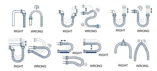
In case the hose snaps off because of its own weight it has to be supported.
